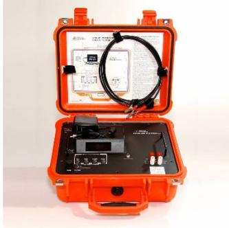
The AMPTEC 620A-4R Igniter Tester was originally designed for U.S. commercial aircraft maintenance, though it's now widely used and trusted by the U.S. armed forces. The 620A-4R contains the same inner circuitry as its ultra-safe predecessor the 620A-4 with the added bonus of protection in harsh environments, an internal Faraday cage for noise immunity, and a wide-viewing angled display. Ready to take on any climate, the 620A-4R is the durable Igniter Tester you've been searching for.
